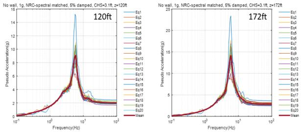
Fig. 5. Response spectra of non-isolated NPP (PGA=1.0g)
