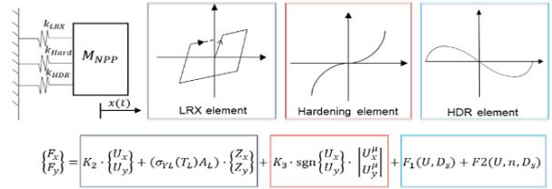
Fig. 2. Parallel numerical bearing model [2]
