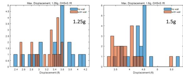
Fig. 8. Effect of moat wall (isolator model: HHHDR, CHS=3.1ft)
