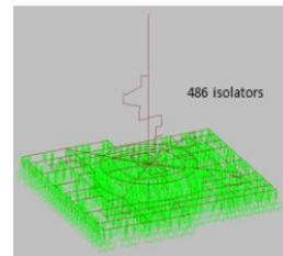
Fig. 4. ANT model with 486 isolators
