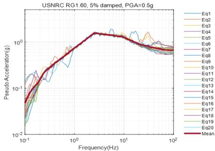
Fig. 1. Pseudo acceleration response spectra of 20 spectral matched motions
