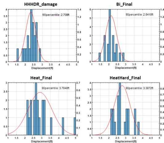
Fig. 7. Maximum displacement distribution (PGA=1.0g)
