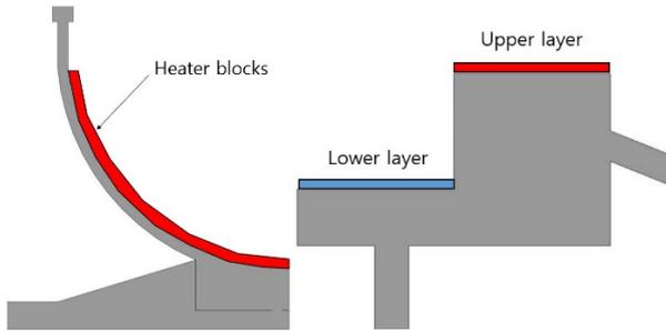
Fig. 3. Heater blocks (left), Condenser (right).
