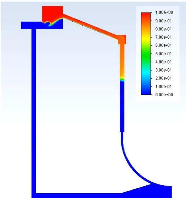
Fig. 6. Liquid volume fraction in the cooling loop; Heat flux=1.233 MW/m<sup>2</sup>
