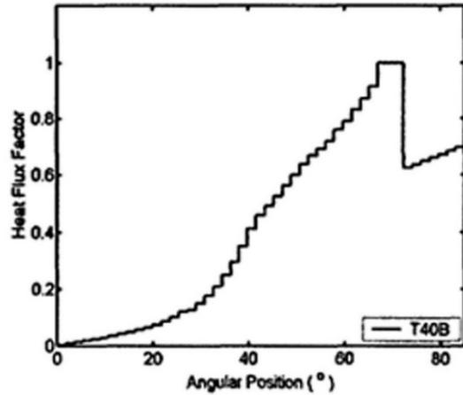
Fig. 4. Angular dimensionless heat flux profile. <sup>7)</sup>
