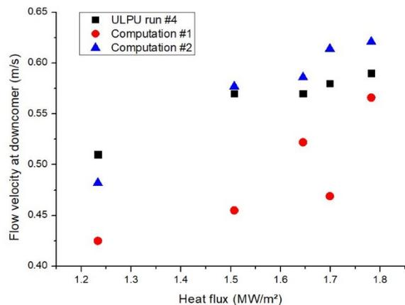
Fig. 5. Comparison of the liquid velocity applying UDF in the downcomer.
