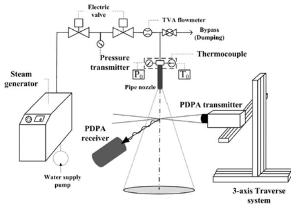
Fig. 1. Layout of a steam jet experiment[4]
