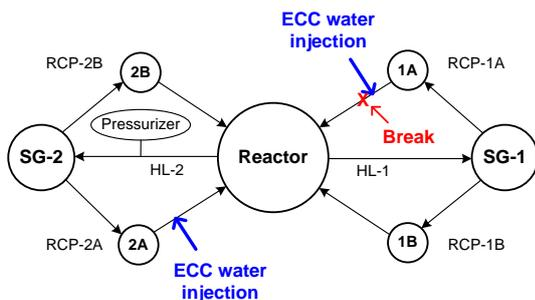
Fig. 1. Location of break unit and ECC injection point [3]
