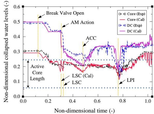
Fig. 4. Collapsed water levels of core and downcomer.
