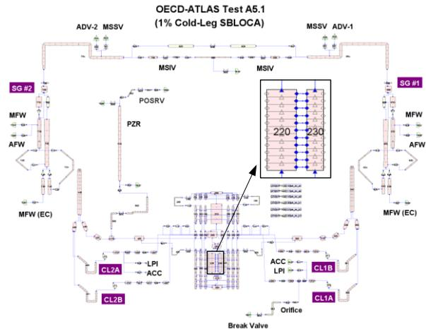
Fig. 2. MARS-KS nodalization of A5.1 test.
