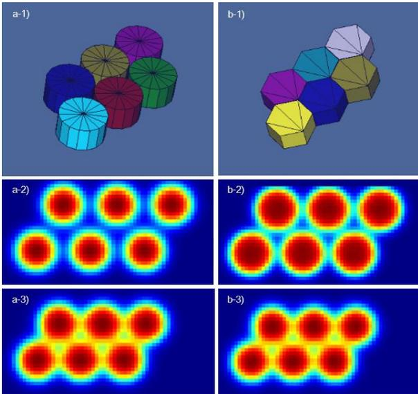
Fig. 3. In MCNP6 simulations, a-1) and b-1) show the 3D shapes of six applicators. a-2) and a-3) show the dose distribution of cylindrical models using  $^{32}\text{P}$ , for wall thicknesses of 2 mm and 0.5 mm, respectively. b-2) and b-3) show the dose distribution of hexagonal models using  $^{32}\text{P}$ , for wall thicknesses of 2 mm and 0.5 mm, respectively.
