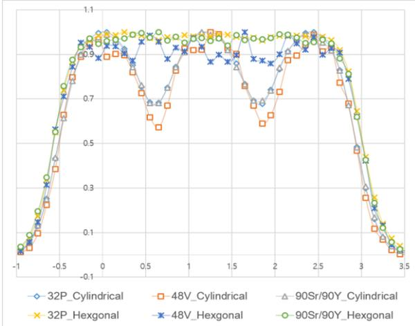
Fig. 2. Trans-axial dose profile of the cylindrical and hexagonal models (0.5 mm wall thickness), for various radioactive sources at a depth of 2.5 mm.
