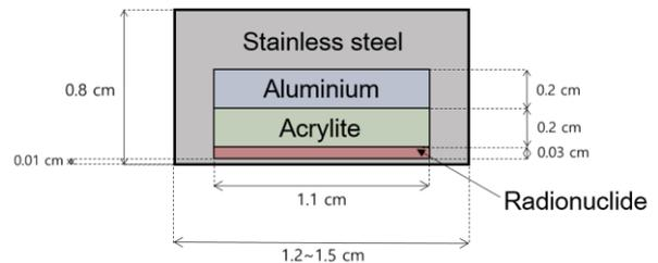
Fig. 1. Schematic (cross-section) of the radioactive module applicator
