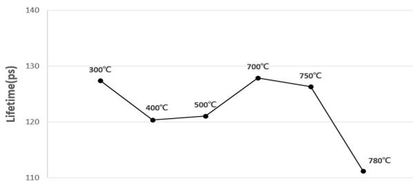
Fig 1. The change according to the temperature applied to hot-rolling was observed as mean lifetime.
