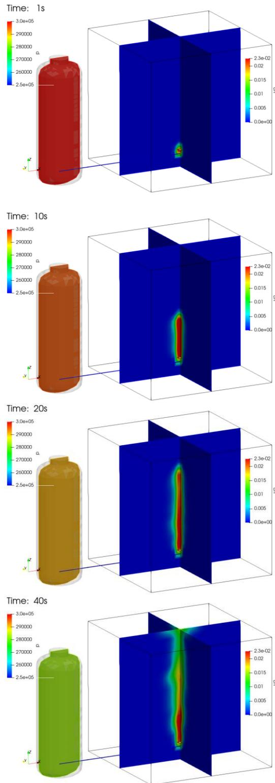
Fig. 2. MELCOR-ContainmentFoam coupled analysis, pressure field in SPARC and hydrogen distribution in the compartment along time.
