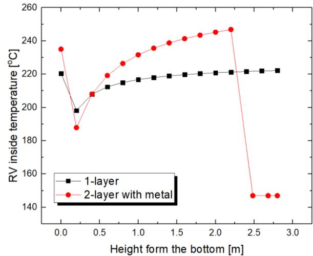
Fig. 3. Temperature inside of the reactor vessel
