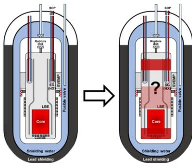
Fig. 1. Schematic of the micro-URANUS and relocation
