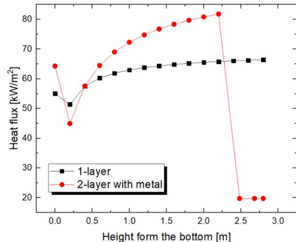
Fig. 4. Heat flux with different vertical position
