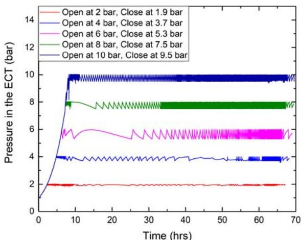
Fig. 5. Change of pressure inside the ECT with various open and close pressure conditions of relief valves.
