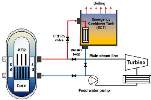
Fig. 2. Schematic diagram of the PRHRS.
