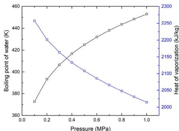
Fig. 1. Boiling point and heat of vaporization of water with pressure.
