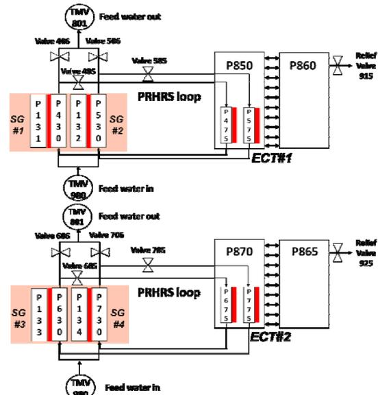
Fig. 3. MARS-KS nodalization of the PRHRS with relief valves.
