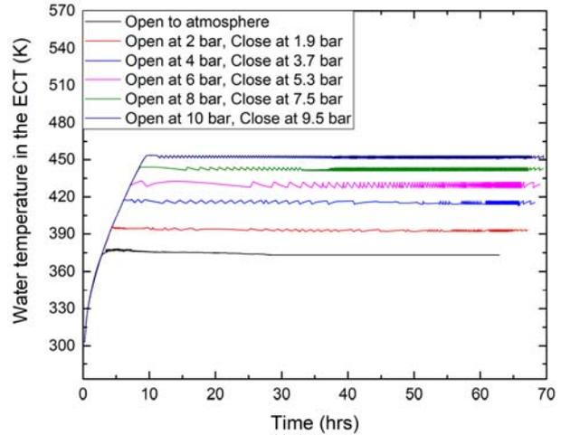
Fig. 6. Change of water temperature inside the ECT with various open and close pressure conditions of relief valves.
