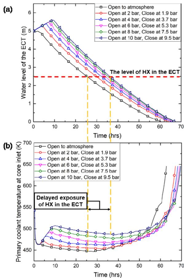
Fig. 7. Comparison of the various open and close pressure conditions of relief valves: (a) water levels of the ECT; (b) core inlet temperature.
