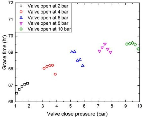
Fig. 4. Effect of the relief valve closing pressure on grace time.
