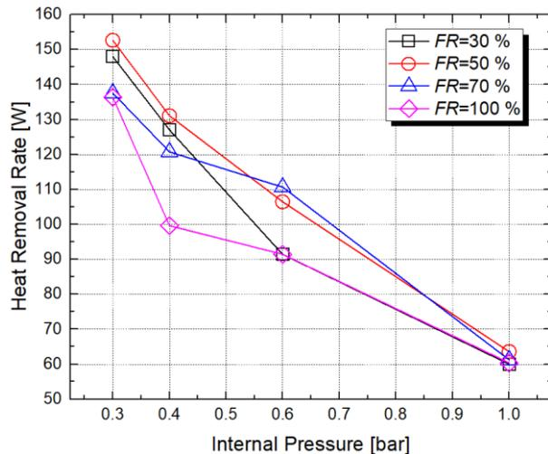
Fig. 5. Heat transfer rates of the hybrid control rod-heat pipe according to internal pressures and fill ratios.
