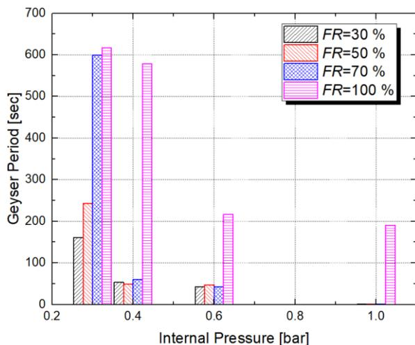
Fig. 7. Geyser boiling periods according to operating conditions of the hybrid control rod-heat pipe.
