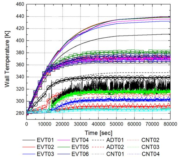
Fig. 3. Basket wall temperature distribution of 1/5 scaled UCAN at steady state ( $Q=1050$  W,  $z=0.455$  m).
