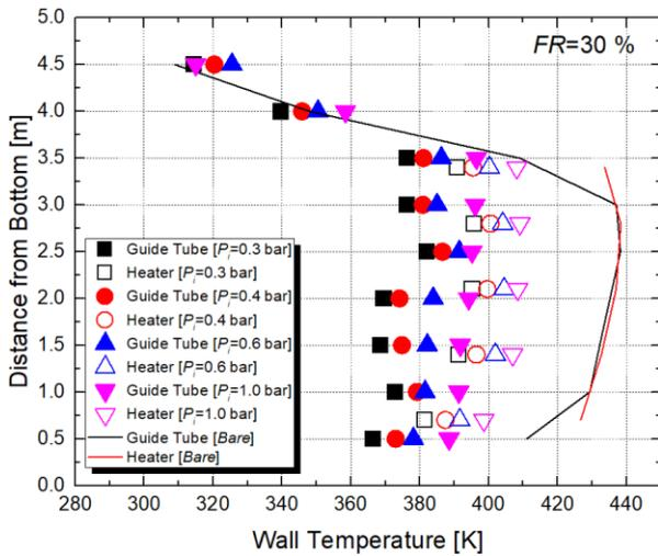
Fig. 4. Comparison of guide tube and heater temperatures according to cask design and operation conditions of the hybrid control rod-heat pipe.
