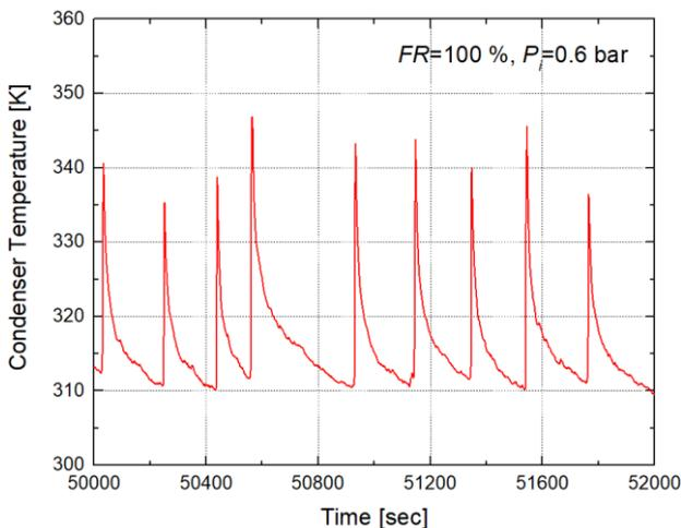
Fig. 6. Wall temperature variation at condenser section of the test section (100 % FR and 0.6 bar internal pressure).
