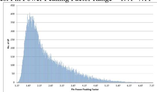
Fig. 3. Pin Power Peaking Factor Distribution (Train)
