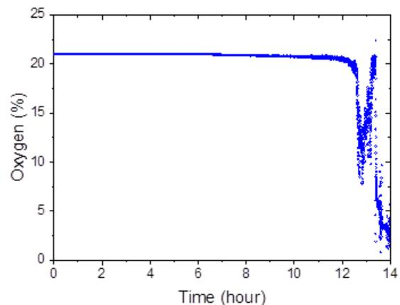
Fig. 2. Fuel assembly oxygen concentration profile with time of the SFP project phase-1 ignition test
