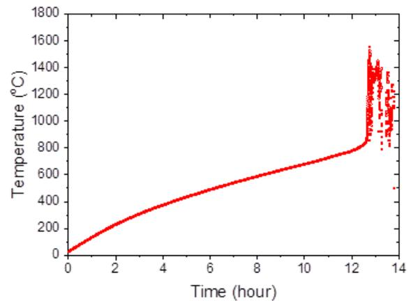
Fig. 1. Fuel assembly temperature behaviors with time of the SFP project phase-1 ignition test
