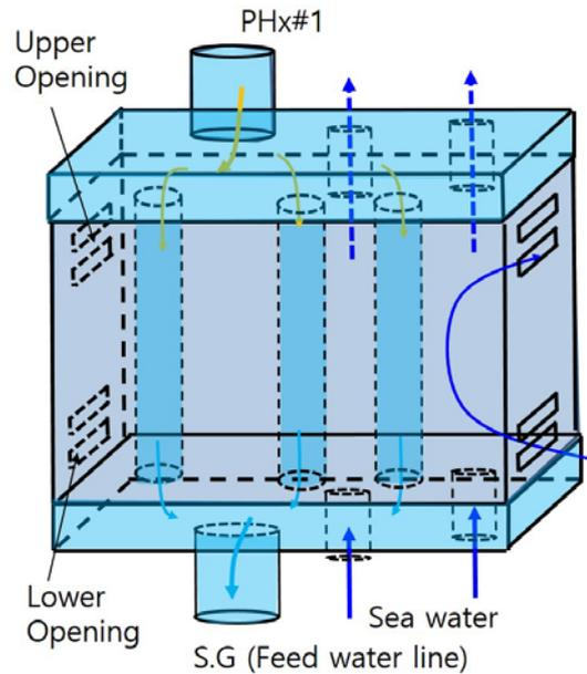
Fig 3. Heat exchanger configuration by sea water
