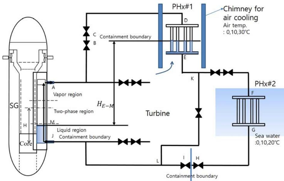
Fig1. Schematic of hybrid residual heat removal system by air and sea water
