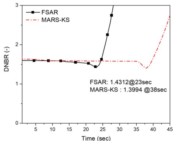
Figure 8. Transient DNBR at the hot pin
