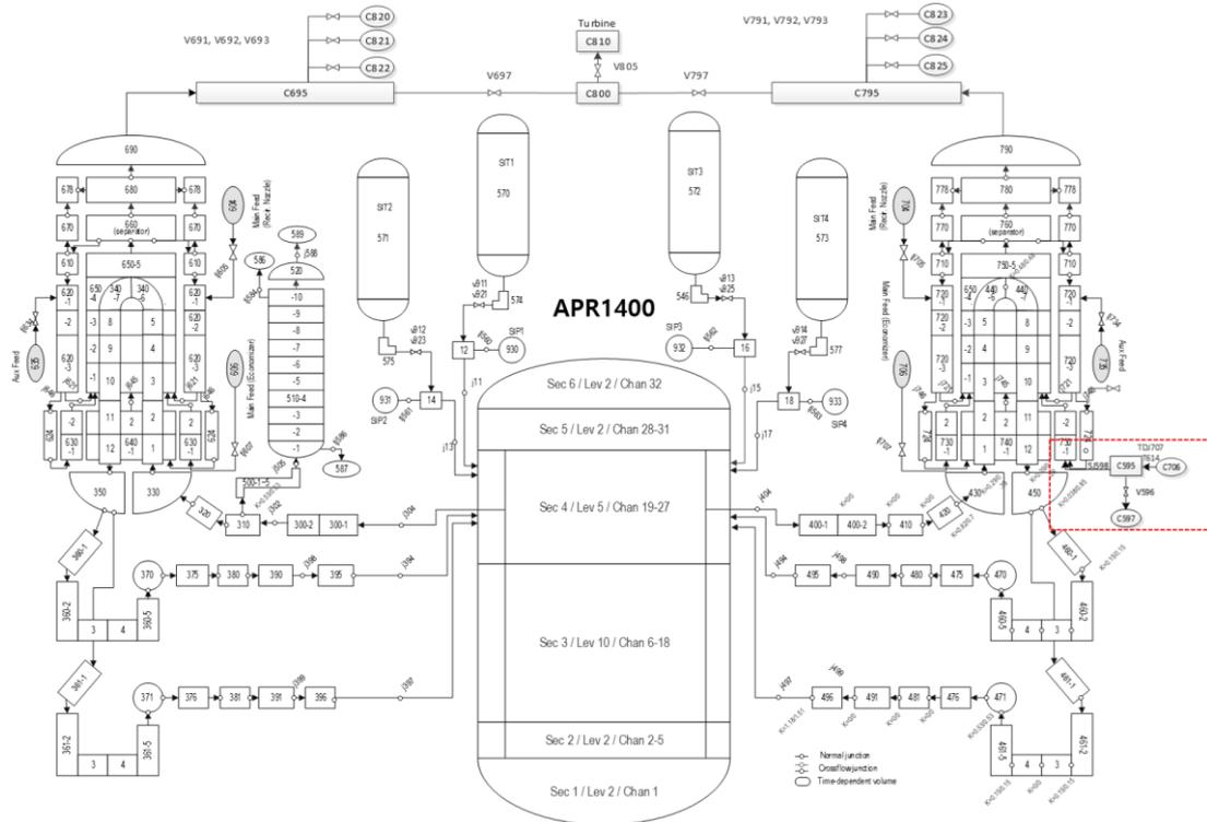
Figure 1. APR1400 MFLB nodalization
