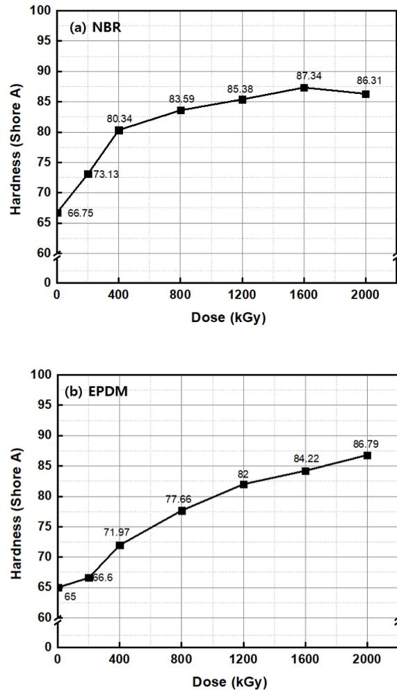
Fig 2. Shore A hardness of gamma irradiated polymer (a) NBR and (b) EPDM
