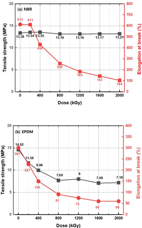
Fig 1. Tensile properties of gamma irradiated polymer (a) NBR and (b) EPDM
