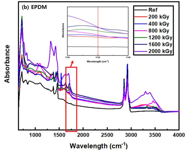
**Fig 3.** FT-IR spectrum of gamma irradiated polymer (a) NBR and (b) EPDM
