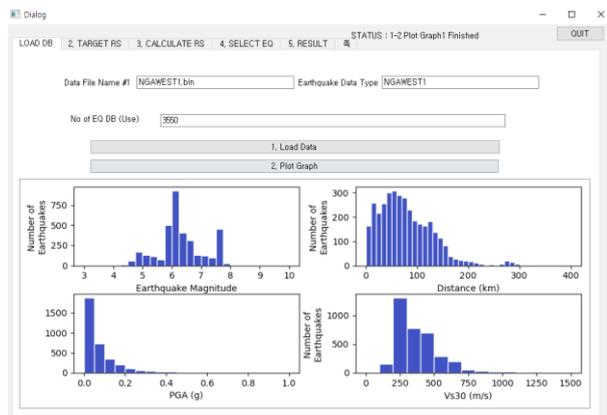
Fig. 3. Screenshot of Load Earthquake Database.
