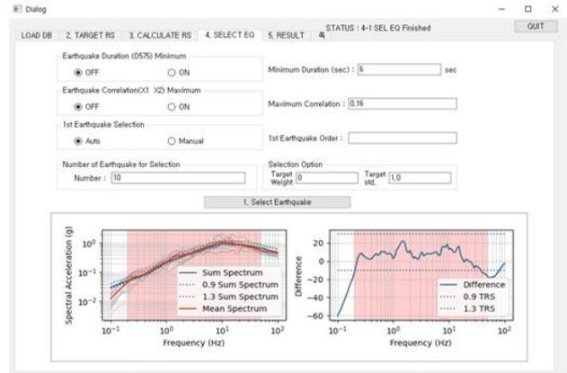
Fig. 4. Screenshot of setting selection option and final results of selected earthquake motions.
