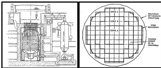
Figure 1. The Calder Hall Reactor Model
