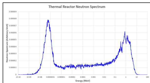
**Figure 4. Neutron spectrum of the thermal reactor**
