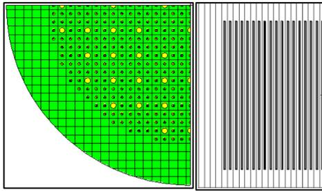
**Figure 2. Quarter core (Left) and the axial core design (Right) of thermal reactor**
