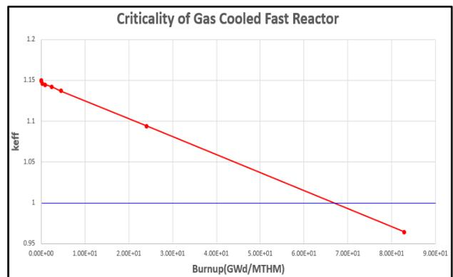
Figure 7. Criticality change of fast reactor
