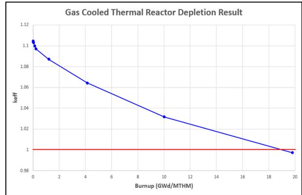
Figure 6. Criticality change of thermal reactor
