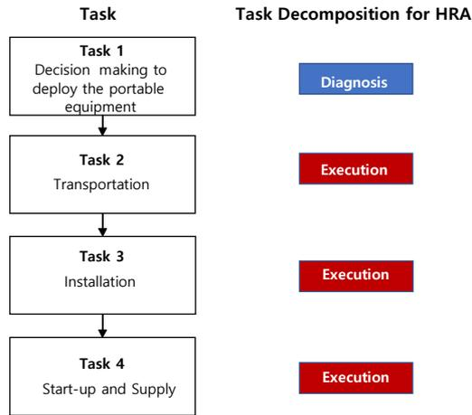
Fig. 1. Task analysis for the HRA of portable equipment
