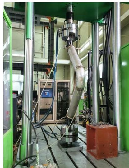
Fig. 2 Setup of failure tests on elbow specimen
