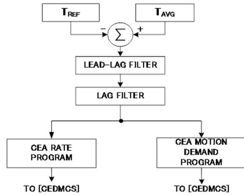
Figure 1. Simplified Block Diagram of RRS
