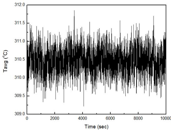
Figure 3. KISPAC Simulation of Steady State  $T_{avg}$  Hunting
