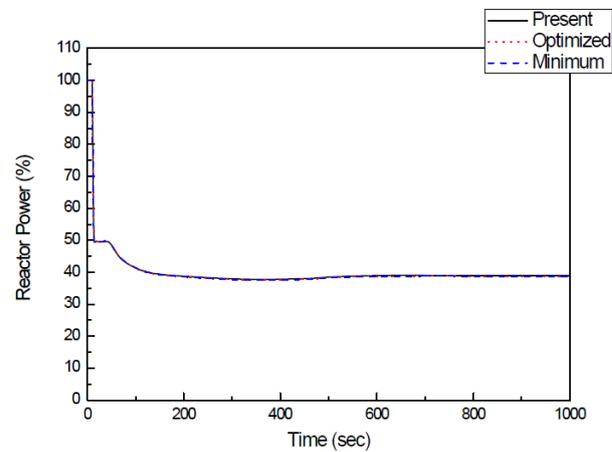
Figure 9. Reactor Power (Loss of a Main Feedwater Pump at 100% Power)
