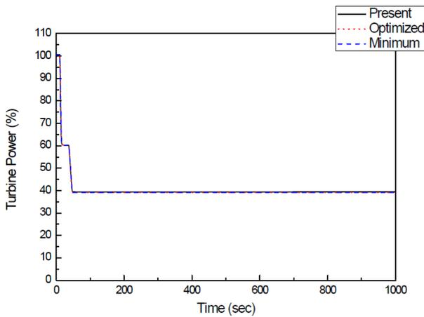
Figure 10. Turbine Power (Loss of a Main Feedwater Pump at 100% Power)
