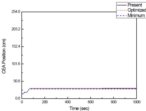
Figure 11. CEA Position (Loss of a Main Feedwater Pump at 100% Power)
