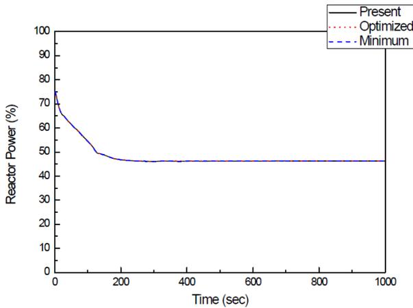
Figure 6. Reactor Power (Load Rejection at 75% Power)
