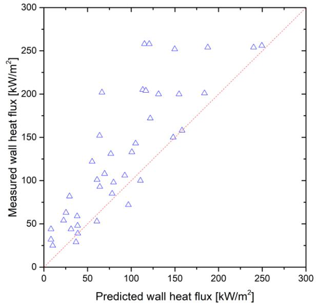
Fig. 4. ONB wall heat flux comparison results.
