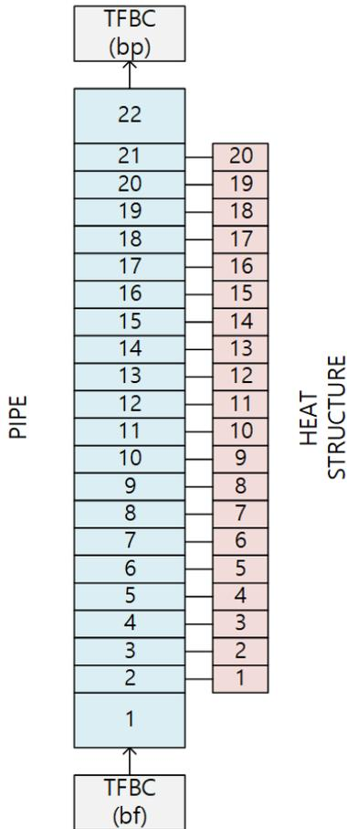
Fig. 2. Code nodalization (not to scale).
