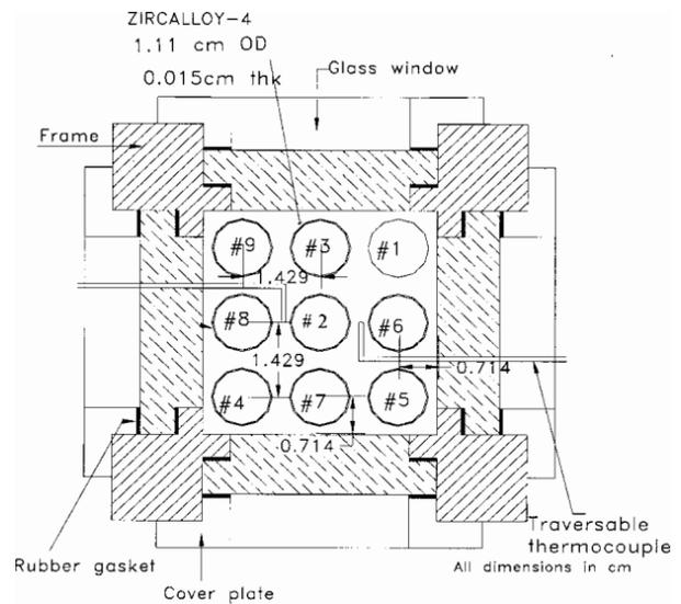
Fig. 1. Cross-section view of the test section (take from [4]).
