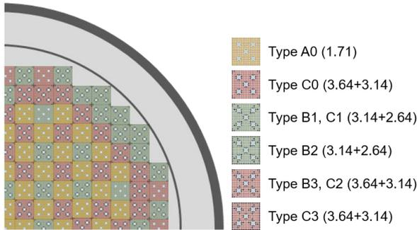
Fig. 3. Radial configuration of APR 1400 quarter core
