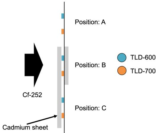
Figure 1. The side view of TLDs of this study.
