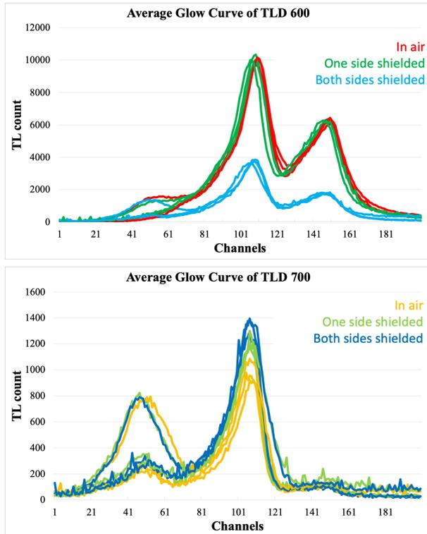
Figure 4. The averaged glow curves of TLD-600 and TLD-700 at three positions.
