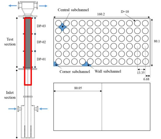
Fig. 1 Schematic diagram of PRIUS-II
