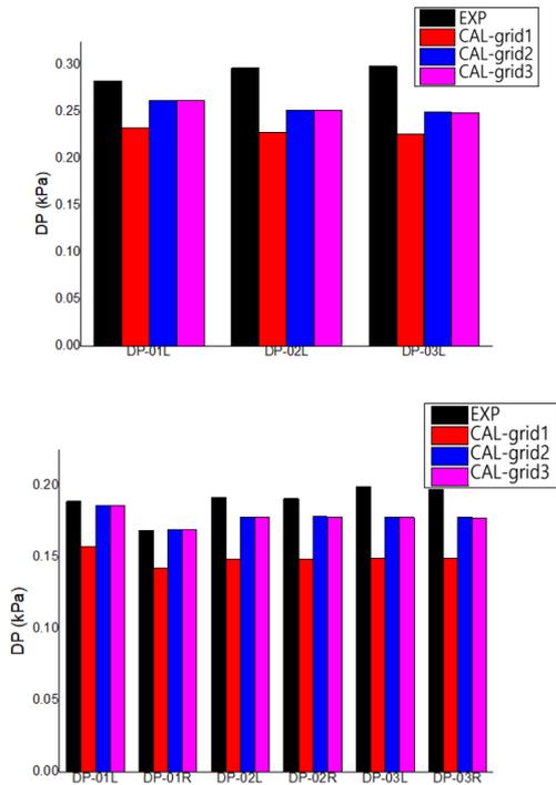
Fig. 3. Grid sensitivity results for water test
