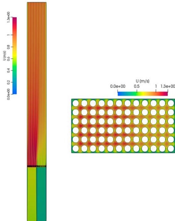
Fig. 4. Preliminary velocity calculation results for a main test (flow rates: 2.164 kg/s, 1.165 kg/s) (left: side view, right: top view)
