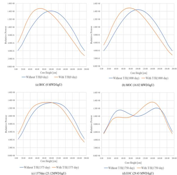
Fig. 7. The comparison results of the axial power distribution
