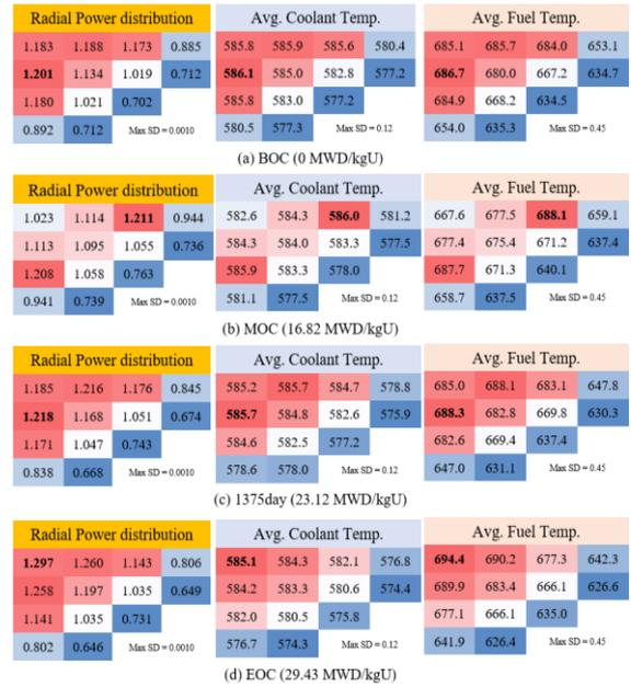
Fig. 6. The radial power distribution and temperature profile calculated with T/H feedback
