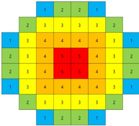
Fig. 2. Loading pattern of SMR
