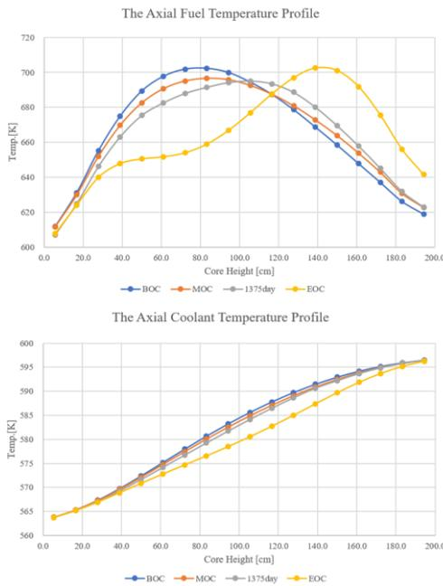
Fig. 8. The axial temperature profile of coolant and fuel
