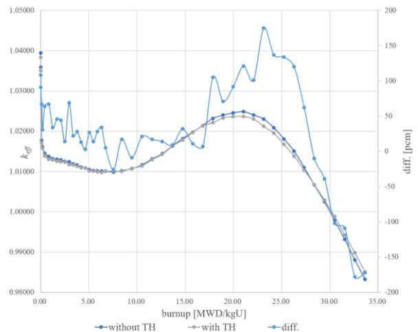
Fig. 4.  $k_{eff}$  vs. burnup behavior with or without T/H feedback
