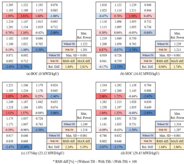
Fig. 5. The comparison results of the radial power distribution
