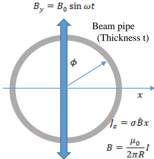
Fig. 2. Magnetic field assumed for eddy current calculation
