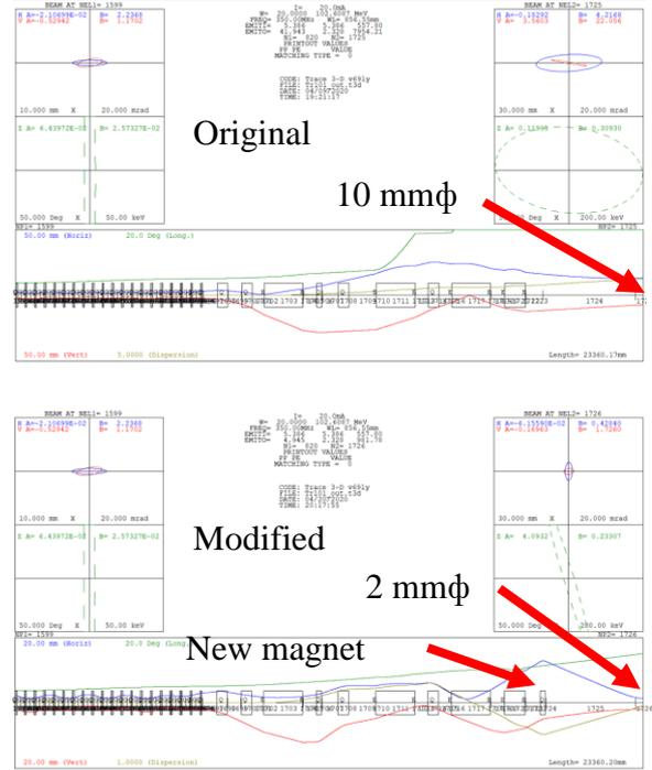
Fig. 1. Beam optics of RI production beamlines
