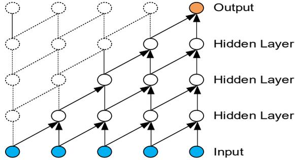
Fig. 2. Visualization of a stack of causal convolutional layers
