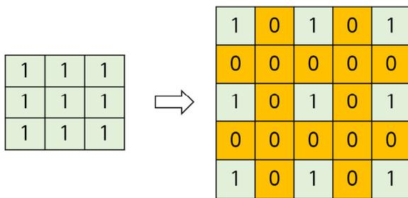
Fig. 3. Conceptual diagram dilation rate in 2-D convolutional layer (Dilation rate=2)
