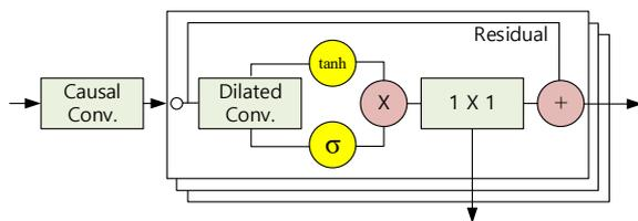
Fig. 4. Schematic Diagram of Gated Activation Unit
