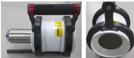
**Figure 2** 45° field of view angle and 2cm thickness collimator for 3inch NaI(Tl) detector
