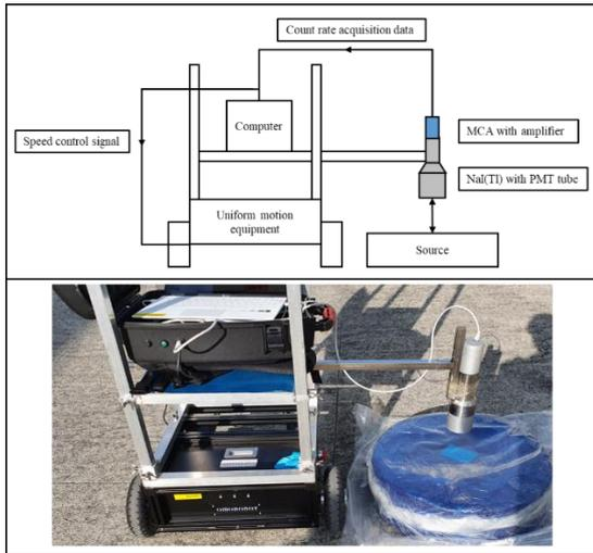
**Figure 1** Uniform motion equipment and scan survey system
