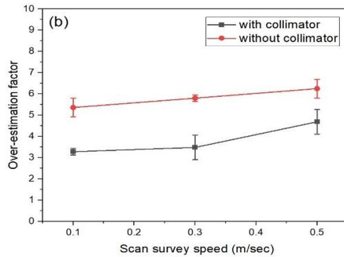
Figure 1 Over-estimation factor change by detector condition and survey speed (a)  $^{137}\text{Cs}$  (b)  $^{60}\text{Co}$
