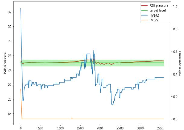
Fig. 3. The change of PZR pressure and valves according to the timestep in the last episode.
