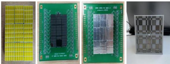
Fig. 3. Components for the coded-aperture imaging system based on 9 of  $4 \times 4$  SiPM array (ArrayJ-30035-16P, On semiconductor) coupled with 9 of  $4 \times 4$  pixels GAGG(Ce) scintillator array partitioned  $3.16 \times 3.16 \times 20 \text{ mm}^3$  pixel and MURA mask (right).
