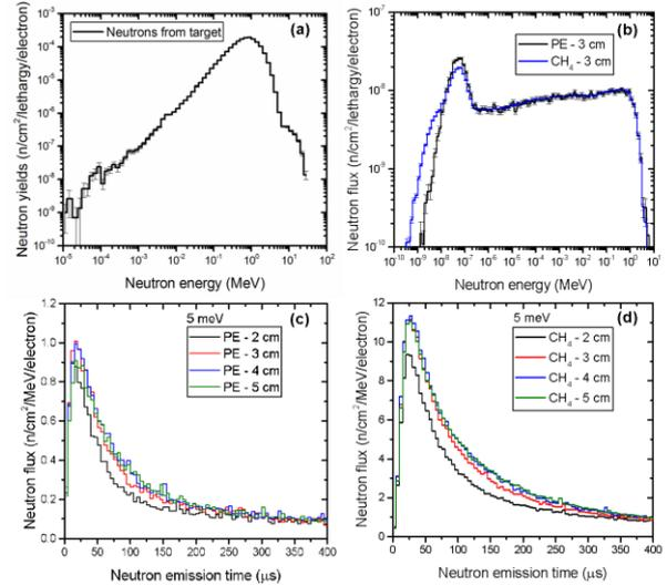
Fig. 3. (a) Neutron spectrum generated in the target, (b) neutron spectra after PE and solid CH<sub>4</sub> moderators at 1 m from the target, (c) neutron time emission for PE, and (d) for solid CH<sub>4</sub>.
