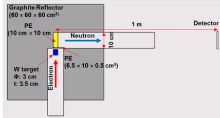
Fig. 2. The target geometry simulated in the PHITS code.
