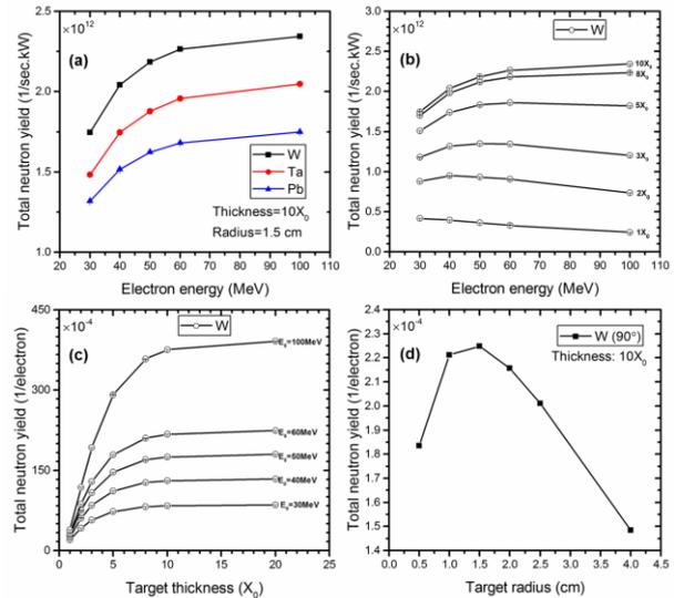
Fig. 1. (a) Total number of neutrons emerging from the targets, (b) variation of neutron yields with electron energy for 1, 2, 3, 5, 8, 10  $X_0$ , (c) neutron yields against W thickness for 30, 40, 50, 60, 100-MeV electrons, and (d) neutron yields against W radius at 90° and  $E_e = 40$  MeV.
