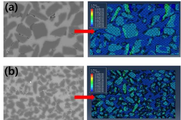
Fig. 5. FEM simulation results of Al/SiC composites with large size reinforcement (a) and small size reinforcement.
