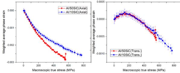
Fig. 4. weighted average phase strain of Al axial (left) and transversal strain (right) of Al.
