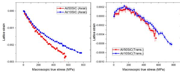
Fig. 3. Axial FCC{311} lattice strain (left) and transversal strain (right).
