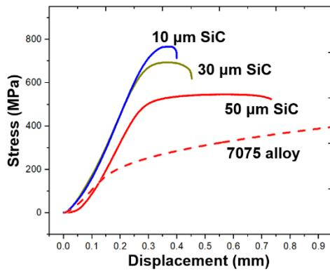
Fig. 2. The compression test results.
