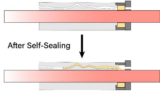
Fig. 2. Example of the self-sealing mechanism
