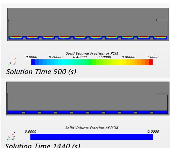
Fig. 9. Solid Volume Variation (Thickness: 20mm, Finned)
