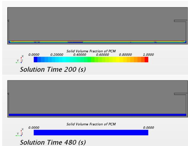
Fig. 7. Solid Volume Variation (Thickness: 10mm, Non-finned)
