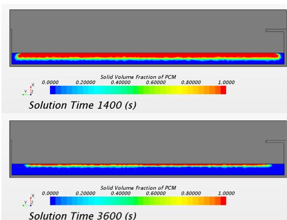
Fig. 12. Solid Volume Variation (Thickness: 40mm, Non-finned)
