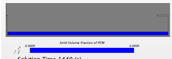
Fig. 8. Solid Volume Variation (Thickness: 20mm, Non-finned)
