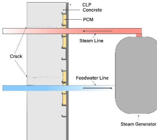
Fig. 1. Diagram of the PCM placed containment
