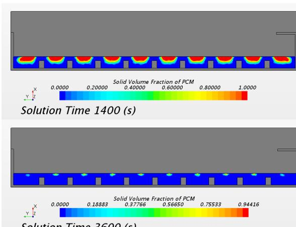
Fig. 13. Solid Volume Variation (Thickness: 30mm, Finned)
