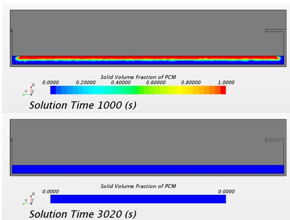
Fig. 10. Solid Volume Variation (Thickness: 30mm, Non-finned)
