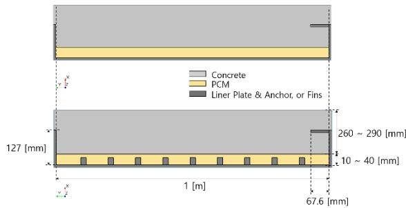
Fig. 4. Geometry scene of the non-finned case (upper) and finned case (lower) (The geometry is 90° rotated in counter-clockwise direction)
