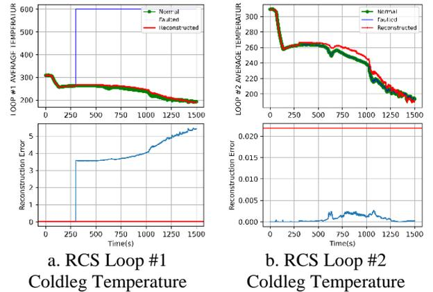
Fig. 4. VAE-LSTM output when stuck at the RCS loop1 Tavg high degrees
