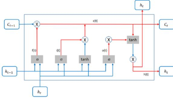
Fig. 2. The architecture of LSTM
