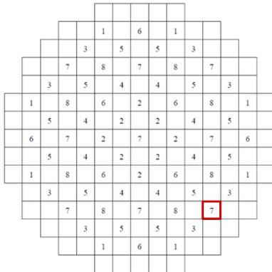
Figure 7. Control rod banks radial mapping and position of the stuck control rod.
