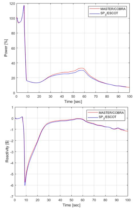
Figure 8. Evolution of power (*top*) and reactivity (*bottom*) during the transient calculated with MASTER/COBRA and the 3D/1D SP<sub>3</sub> code coupled with ESCOT.
