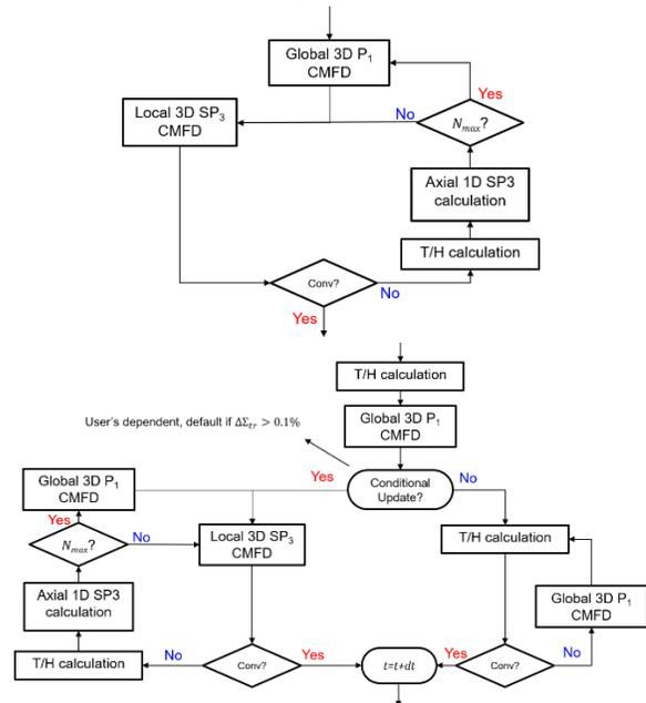
Figure 1. Calculation flow for the 3D/1D based SP<sub>3</sub> code, steady-state (*top*) and transient (*bottom*).
