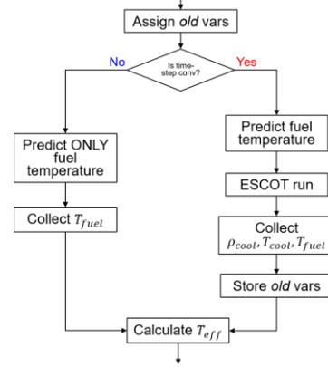
Figure 4. ESCOT interface for the transient coupling.
