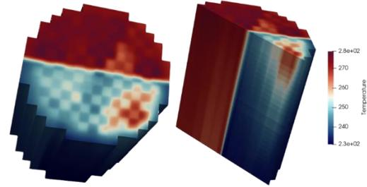
Figure 11. Coolant temperature distribution at 57.0 seconds.
