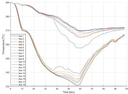
Figure 6. Evolution of the inlet coolant temperature for the eighteen core sectors.
