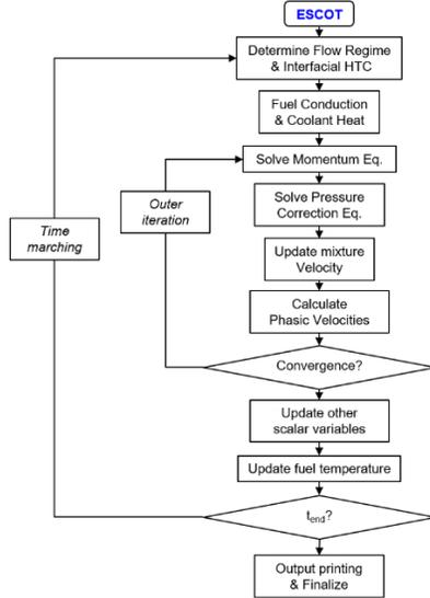
Figure 2. ESCOT code calculation flow for transient simulations.
