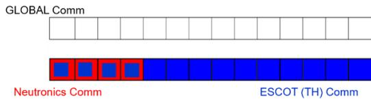
Figure 3. Coupling topology between the neutronics solver and the ESCOT code.
