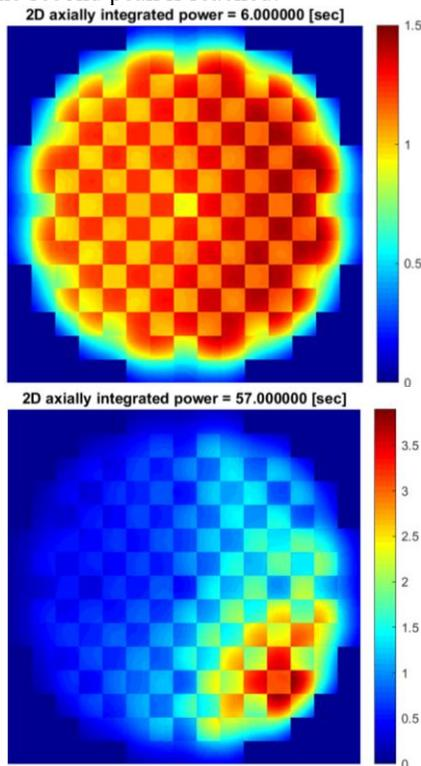
Figure 10. 2D axially integrated power measured at 6.0 (top) and 57.0 (bottom) seconds.
