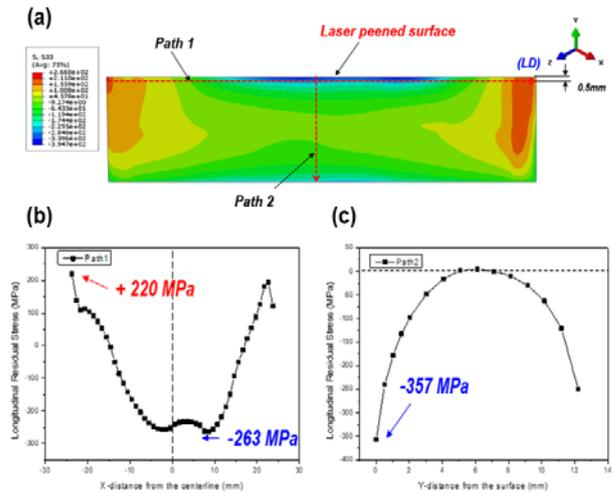
Figure 5. a) Longitudinal residual stress, b) Path 1, c) Path 2
