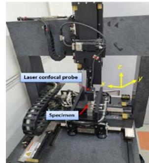
Figure 2. CM measuring equipment by KAERI
