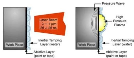
Figure 1. The mechanism of laser peening device [2]
