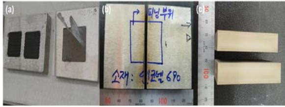
Figure 3. a) Laser peening, b) WEDM cutting, c) A pair of cut surface
