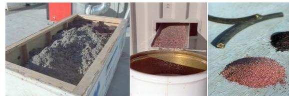
Fig. 7. Final product using recycling cable system (dust, insulation and copper) [5]
