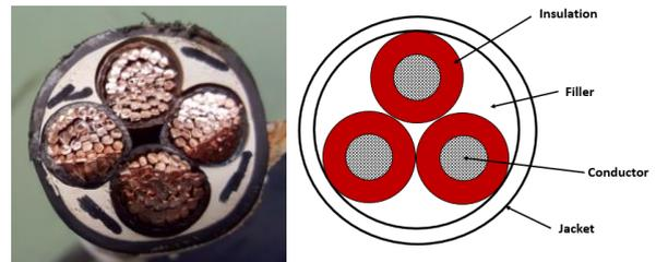
Fig. 2. Cross section of cable and structure of cable [1]
