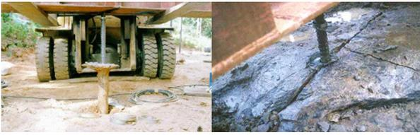
Fig. 2 Rock-grout bond failure (Highly weathered, depth=1.0m) Fig. 3 Rock failure (Moderately weathered, depth=2.0m)
