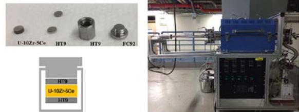
Fig. 1. Schematic diagram of the holder and furnace
