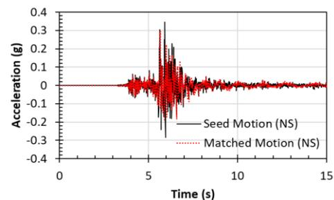
Fig. 2. Acceleration time histories for seed ground motion and spectral matched ground motion.
