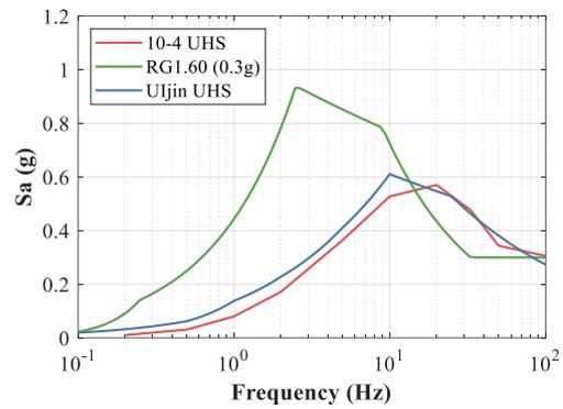
Fig. 1. Uniform Hazard Spectrum for LILW Disposal Facility Site
