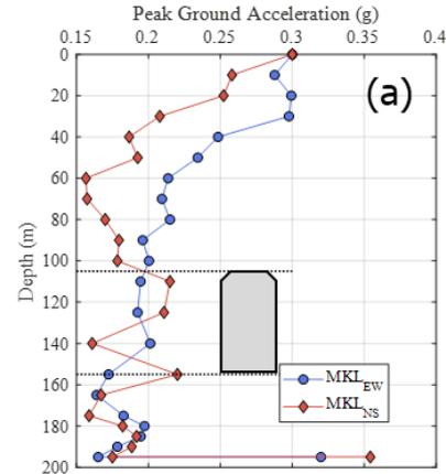
Fig. 4. Peak Ground Acceleration Profile from Site Response Analysis
