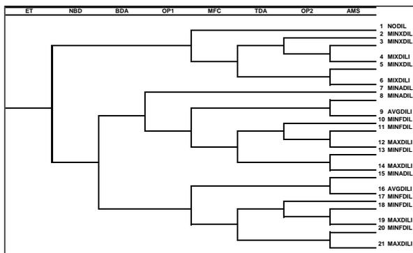
Fig 1. Event Tree for Determining Reactor Makeup Initiating Event Frequency
