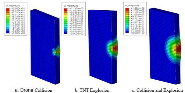
Fig.4. Collision and Explosion FE Analysis
