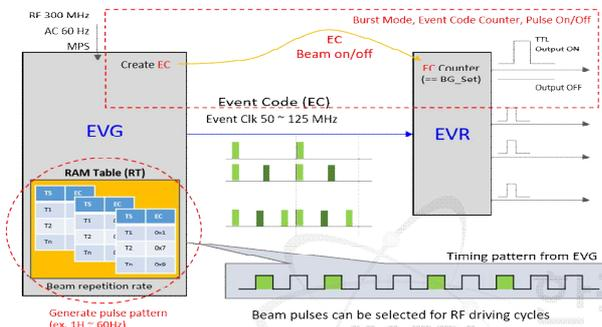
Fig 4. Timing patterns for accelerator operation are generated using sequence ram of EVG and transmitted to EVR
