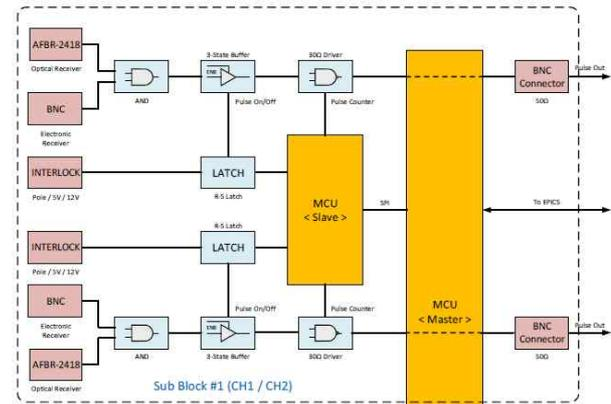
Fig 6. Schematic diagram of beam counter system
