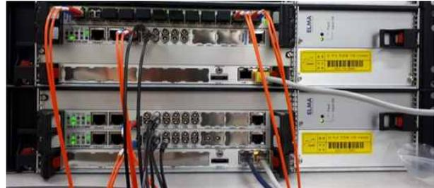
Fig 1. MRF timing system EVG EVR and fan-out
