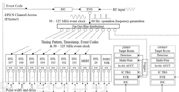
Fig 2. Schematic layout of the event timing system in the klystron galley and beam experiment hall.
