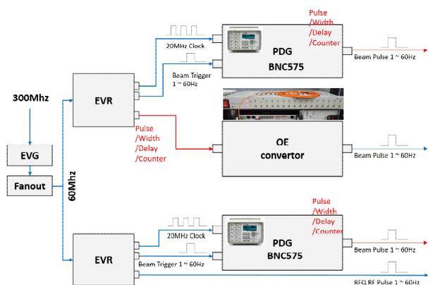
Fig 3. Schematic for providing beam triggers to an injector and beam target rooms using timing system and pulse delay generator.
