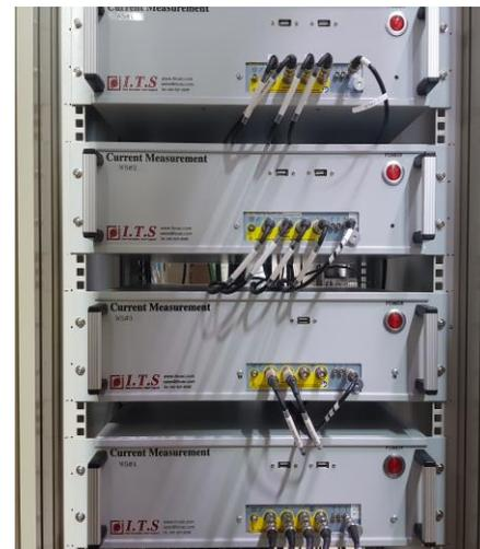
Fig. 3. The wire scanner control units installed in KOMAC beamlines.
