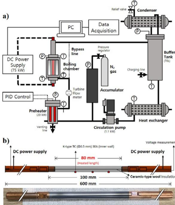
Fig. 2. Schematic diagram of (a) forced convective flow boiling test loop; (b) test section.
