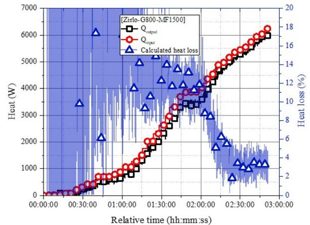
Fig. 3. Comparison of input and output power and calculated heat loss in the test section following the test time.
