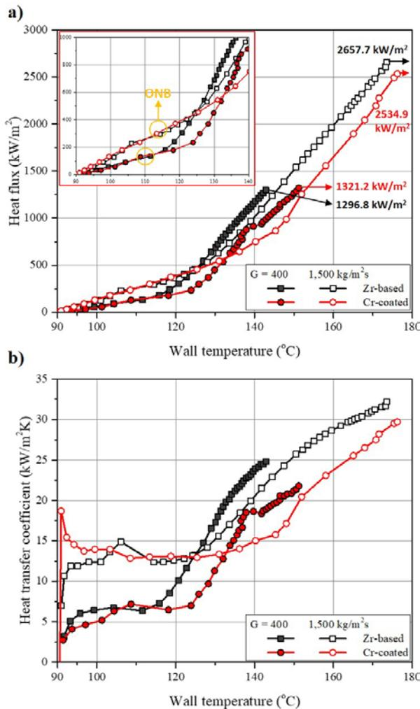
Fig. 5 (a) Boiling curves and (b) heat transfer coefficient of water for tested tubes at the fixed flow conditions (10 °C inlet subcooling, 0.131 MPa, and 400&1,500 kg/m<sup>2</sup>s).
