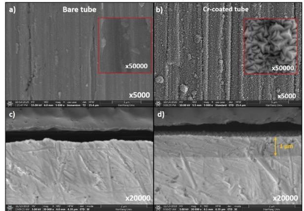
Fig. 1. SEM images of surface morphology on (a) bare tube and (b) Cr-coated tube and cross-sectional images (c) before and (d) after deposition of Cr layer.
