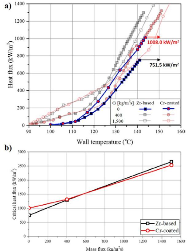
Fig. 4. (a) Boiling curves of Zr-based and Cr-coated tubes at saturated pool boiling condition.; (b) Comparison of measured CHF values following the mass flux condition.
