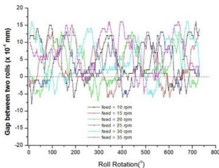
Fig. 4. Gap between two rolls according to the change of feeding speed.
