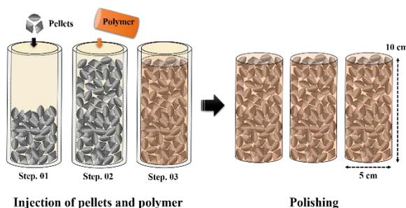
Fig. 1. Manufacturing process of polymer solidification.
