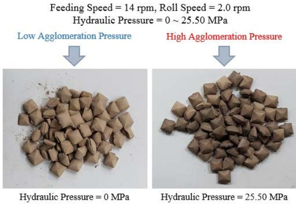
Fig. 2. Manufactured pellets according to change of hydraulic pressure.
