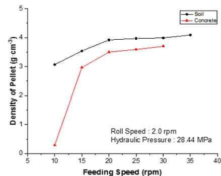
Fig. 6. Change of density of pellet according to feeding speed.
