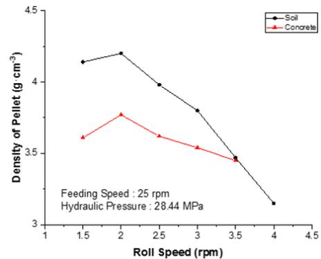
Fig. 5. Change of density of pellet according to roll speed.
