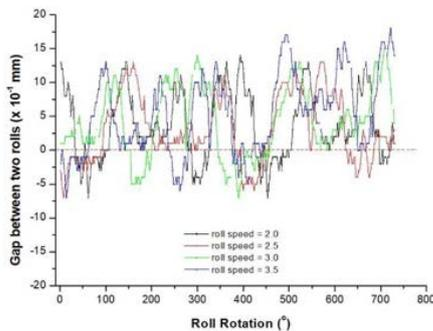
Fig. 3. Gap between two rolls according to the change of roll speed.
