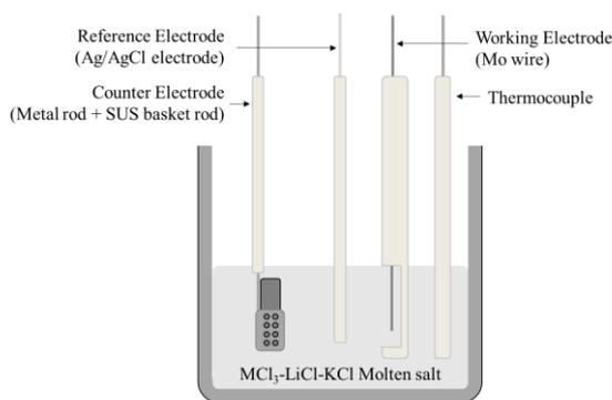
Fig. 1. Electrochemical cell design for the experiment
