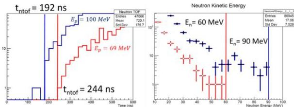
Fig. 4. Neutron time-of-flight histogram and processed energy histogram at 69 MeV and 100 MeV proton beam experiments
