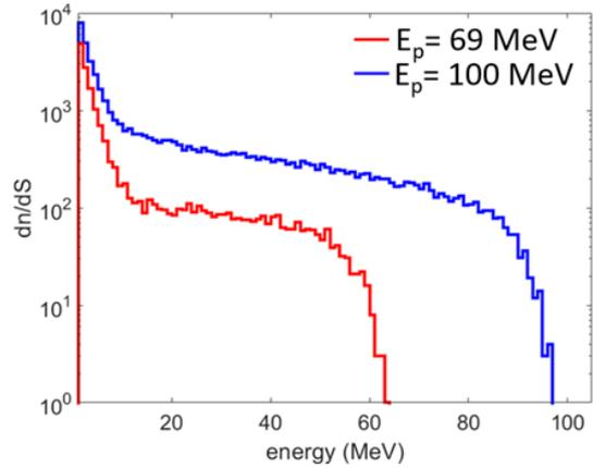
Fig. 5. Neutron energy spectra calculated by Monte-Carlo simulation.
