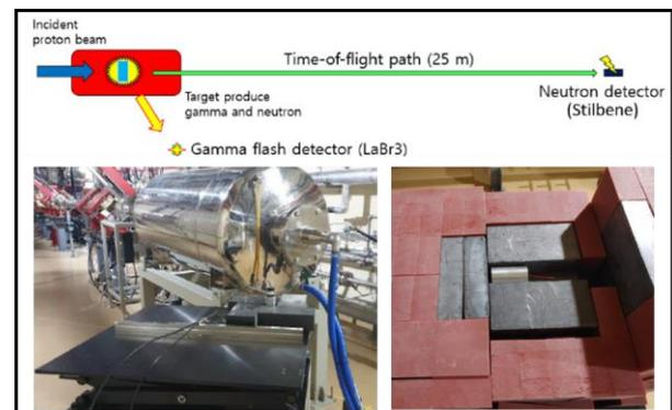
Fig. 2. Overview of gamma-flash tagging neutron time-of-flight measurement.
