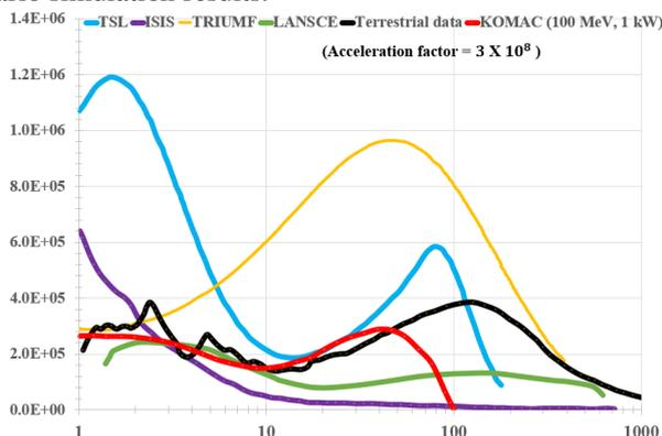
Fig. 1. Lethargy representation of white neutron sources and terrestrial neutrons [1,2].
