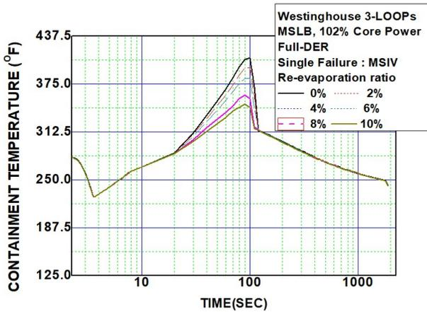
Fig. 3 Containment Temp. in each re-evaporation rate
