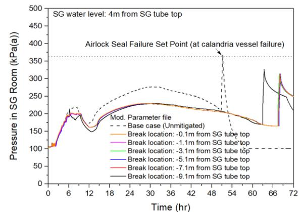
Fig. 4. Pressure transient in the reactor building according to break location during MSGTR.
