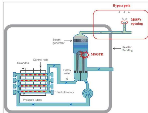
Fig. 1. Reactor Building Bypass Route due to MSGTR [3].
