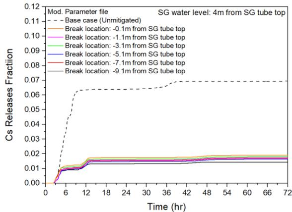
Fig. 5. Cs fraction released to environment according to break location during MSGTR.
