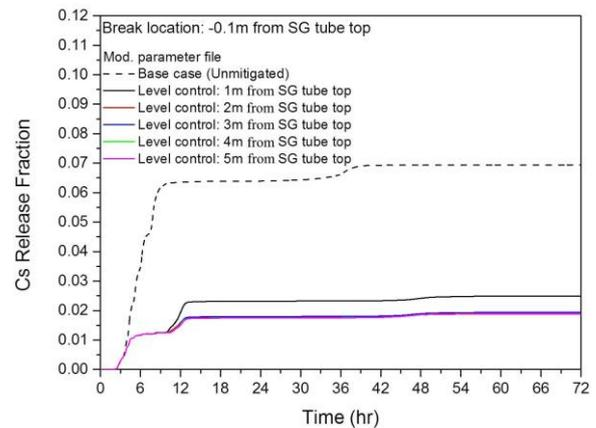
Fig. 3. Cs fraction released to environment according to SG water level during MSGTR.
