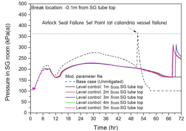
Fig. 2. Pressure transient in the reactor building according to SG water level during MSGTR.
